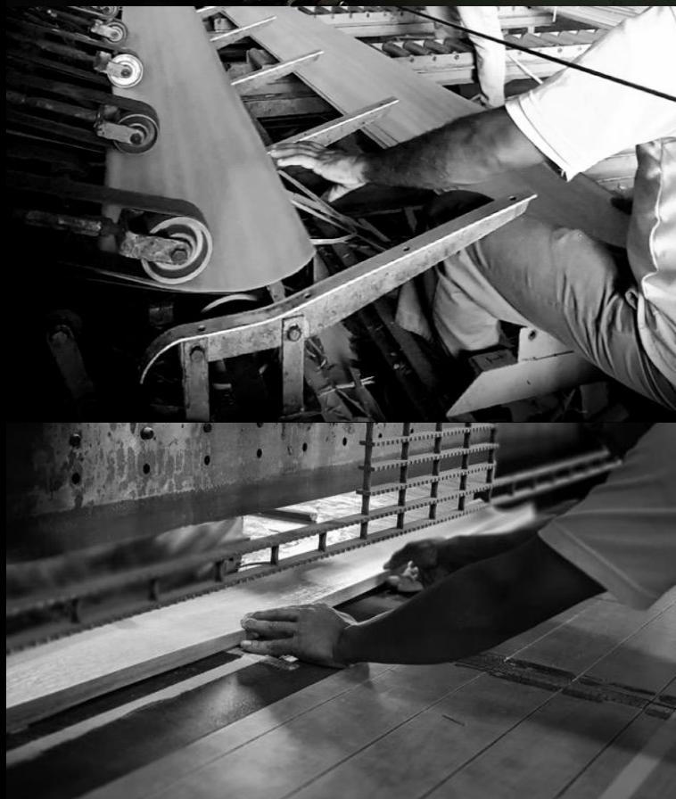
Laser light guided flitching facilities
